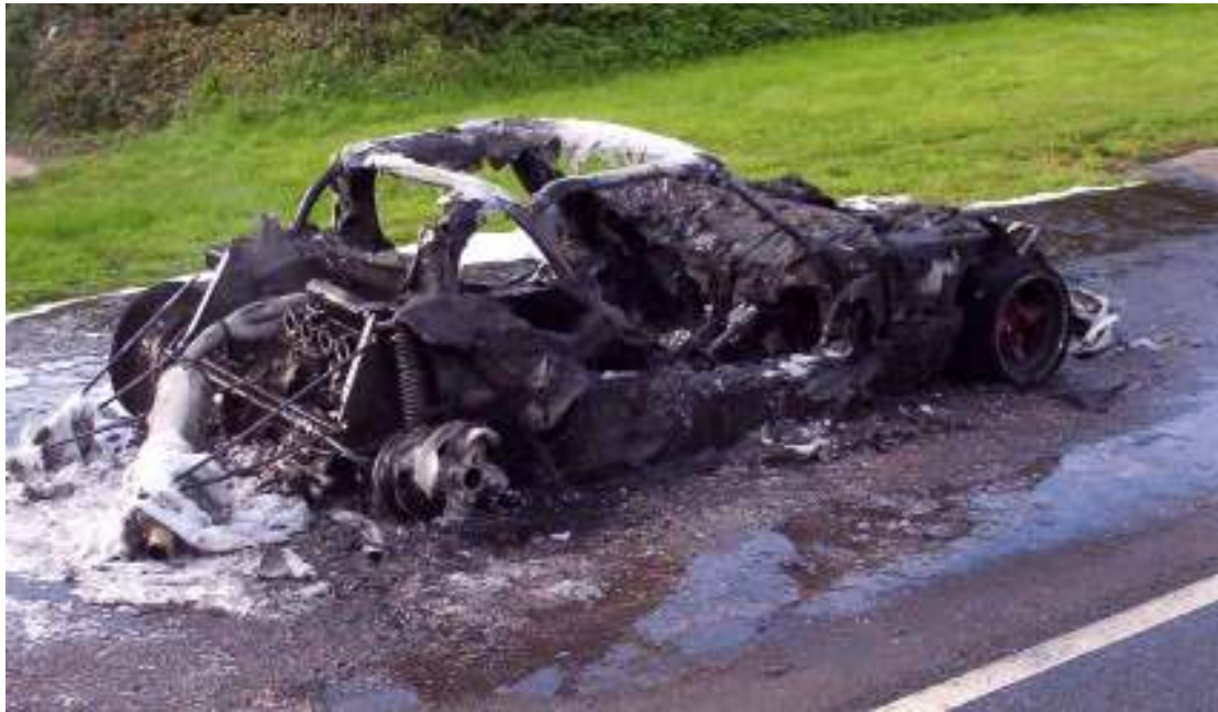
Accidents can happen, but are very rare. The driver emerged from this Darrian sports car uninjured after the engine blew and caused petrol to leak onto a hot exhaust. This accident happened at a test session.
