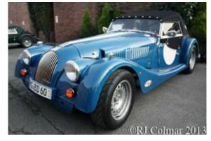
The road legal Baby Doll VI is fitted with a race tuned 225 hp 2 litre Duratec motor, Omex racing clutch, Tillet FIA racing seats, 4 point race harnesses, fire extinguisher, alloy Roadster wheels and Yokohama tyres.
