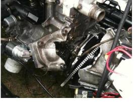
On removing the engine and taking apart what was left we found we needed: Flywheel, Engine Block, Gearbox casing, Starter Motor, Clutch, Gearbox Input Shaft, Head-work and Crank to name a few bits. Most of these items have been replaced and work is on going on the major parts. We are hoping to have the engine and gearbox back together in the next month ready for testing before the season starts again in April once again at Snetterton.
