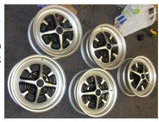
time to dry. I then flatted back with 1200 grade wet and dry, before polishing with cutting compound, T cut and Autoglym. Any small marks were touched back in with a model making airbrush attached to the compressor to avoid buying expensive tins of air. The finished result may not be perfect but I am happy enough with it.
