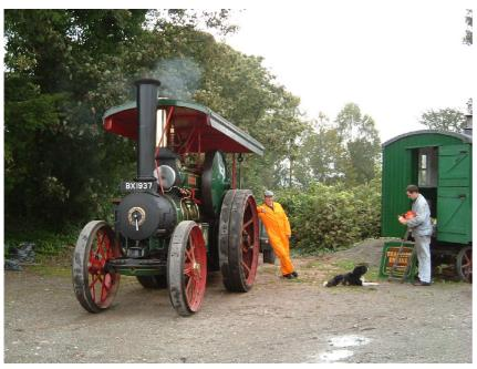
Photograph: The author (complete with Dibnahesque flat cap) leans on the driving wheel of Western Star, Muncaster Castle car 11/09/2004. park, The smokebox is immediately below the number plate, and the low-pressure (large bore) cylinder is visible to the right of the chimney, which conceals the highpressure one. Note the size of the flywheel! On the right, Chris Harrison and dog. (Photo by P Goodman)
