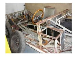
It was then dipped (flowing up the inside of the tubes), painted and Waxoyled and will outlive all of us. The Chevrolet engine was in a poor state having also been 'improved' in the past and was completely rebuilt by Mike Huddart at Huddart Racing Engines, builder of a number of historic race winning motors. The Warner T10 gearbox was rebuilt by Competition Transmission Services and the Salisbury LSD (per E Type Jag) by Alan Slawson at AJS Engineering.
