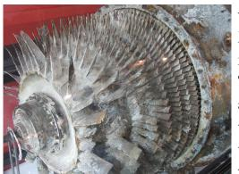
working order. Bill Smith, who recovered the boat in March 2001, has been leading the restoration, utilising as much of the original structure as possible, at his North Tyneside workshop. Luckily much material was intact and could be salvaged due to depth and cold, stable water temperature in the lake. Also, the magnesium casing of the Bristol Siddley Orpheus engine appears to have worked as a sacrificial anode, preventing much worse
