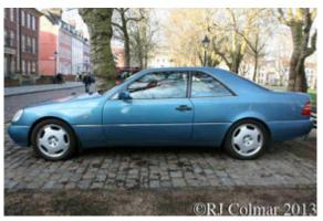
The CL could be ordered either with a 5 litre V8 known as the CL 500, or a 6 litre V12 known as the CL 600. The CL 500 is considered to be the better car because the motor was both lighter and shorter which improved both weight distribution and consequently handling.
